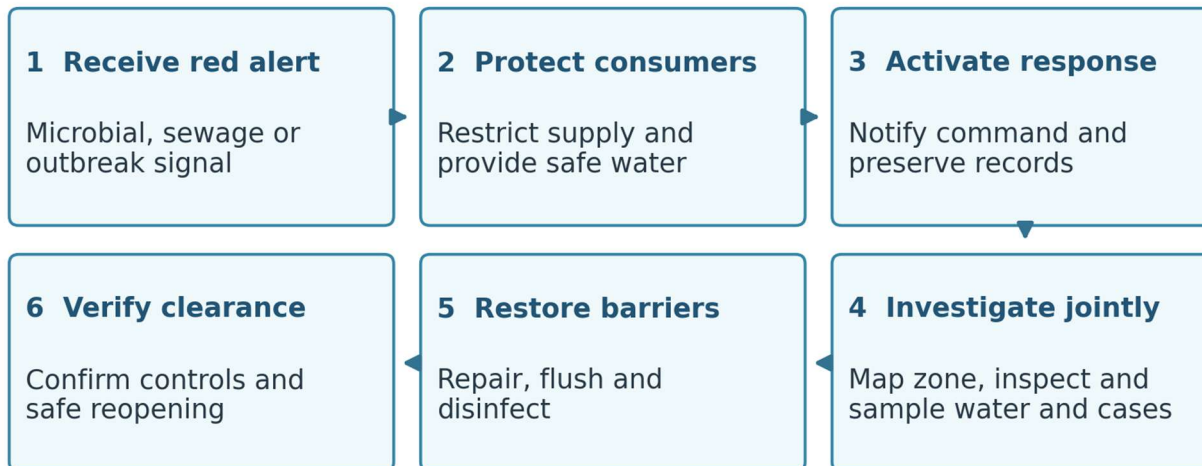
Figure 3 Response to a critical water quality alert
