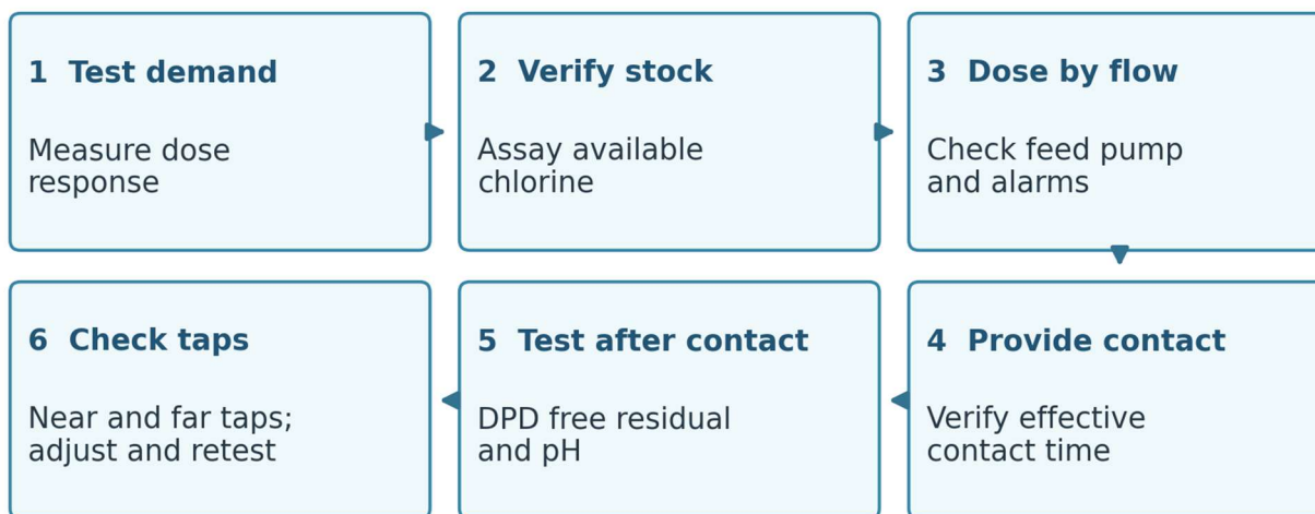
Figure 2 Chlorine dose contact and residual control
